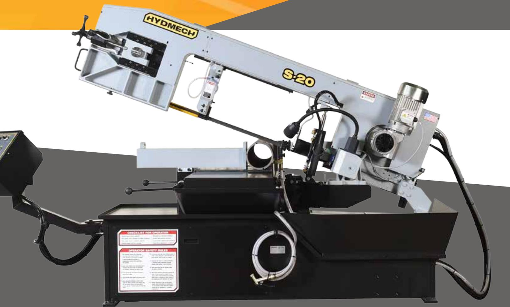
The S-20 represents the first band saw to incorporate a swing head design for miter cutting. The innovative design saves operator set up time and shop space. These versatile machines provide exceptional miter cutting for light to medium duty applications.
