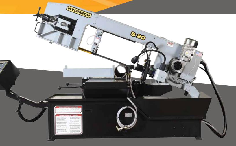
The S-2O represents the first band saw to incorporate a swing head design for miter cutting. The innovative design saves operator set up time and shop space. These versatile machines provide exceptional miter cutting for light to medium duty applications.
