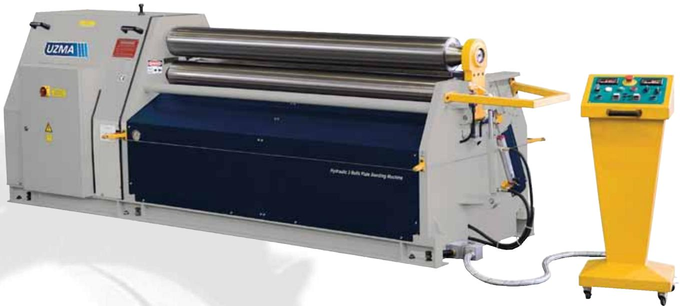
This hydraulic model is designed for light to medium jobs. It is used in jobs up to 10 mm thickness materials. It is used in Aluminium Bendings, Air Conditioning Channels, Advertising Panels and Machine Sheet Metal Cover Parts.
