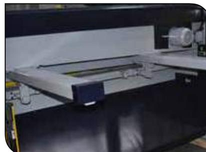
• The MG line Mechanical Shears are Standard with 750mm motorized ball screw back-gauge.
