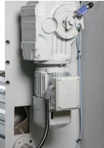
Twin motor drives for the folding contribute both speed and a high degree of accuracy.
