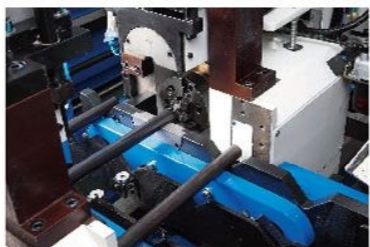
Double Tube Ends Chamfering + Length Measuring ( FM-76V )
