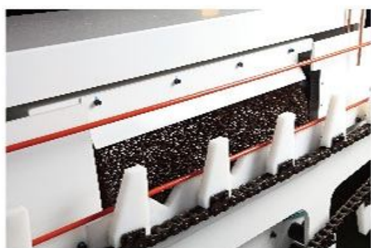
V Shape Guide Way for Square and Rectangular Tubing ( BDB-70 )
