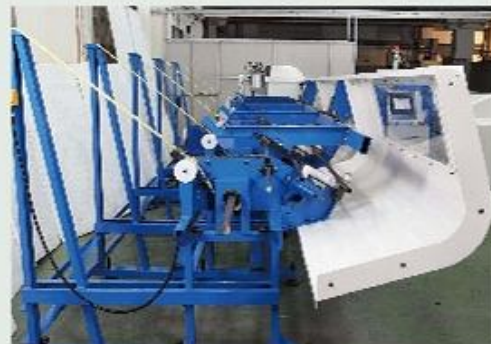
Bundle Loading Magazine. For Tube Length up to 6.5 / 8.5 / 12.5 meters
