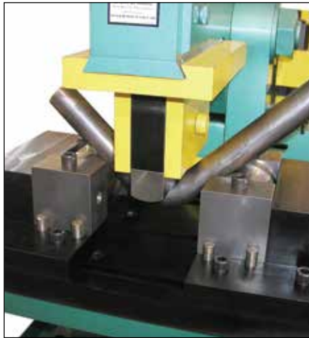
Adjustable bending attachment for solid round bar. Used for non-scaff bending of anchor bolts.
