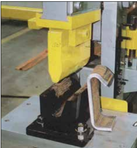
Bending attachment for acute angle bending of flat bar.
