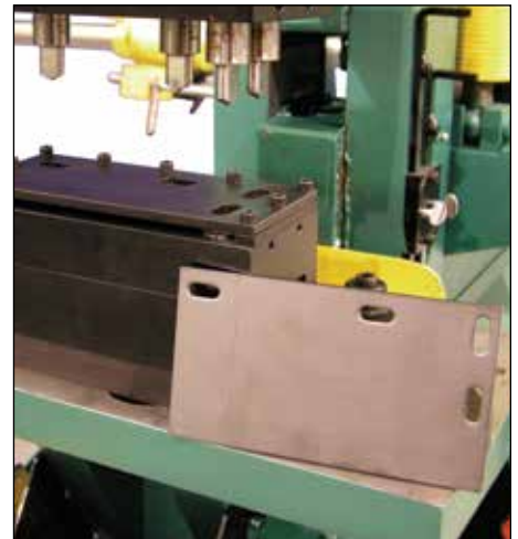
Multiple hole punch. Equal force applied though each punch.
