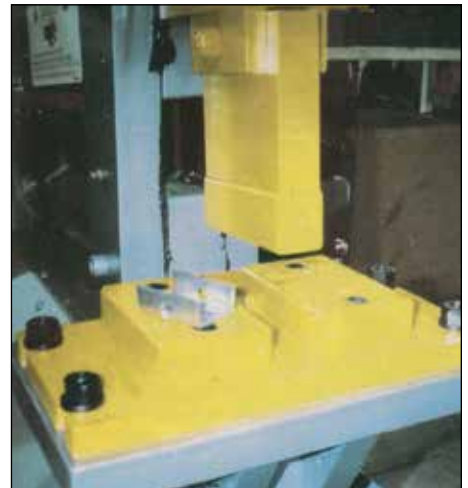
Convertible "U" bracket bending attachment. Capable of bending different "U" widths using the same base.
