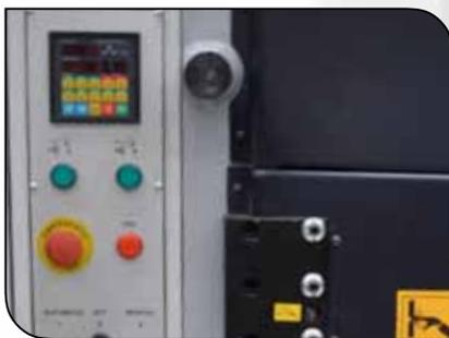
• The MG line Mechanical Shears are Standard with NC control which provides "multi-step" and "touch and go" programming features for the backgauge.
