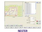
Automatically nest parts on a specified sheet size from the Shape Library or custom CNC files saved on the hard drive. NESTER can even nest parts on
