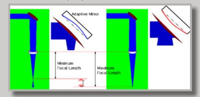
This pneumatic-control AFC adaptive optical system keeps the focused beam spot size constant and consistent wherever the cutting head is located; also providing the pre-programmed automation of focal positioning when loaded with a different material
