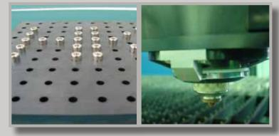
The innovated Quick Pierce System is a built-in standard feature which makes piercing for thick materials swift and effortless; which makes the hole 50-60% in diameter of the thickness that will appear as a pulse pierce, making the hole miniscule & clean.
