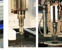
**PNEUMATIC & ELECTRIC DRILLS** Drill up to 3/8" diameter holes in mild steel and 5/16" diameter holes in aluminum with one half HP. Can be combined with normal plasma and oxyfuel cutting, allowing less material handling to be done on the piece part. (Optional)
