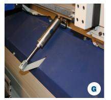
**DAMPER CONTROL DOOR** Programmable pneumatic cylinder actuates the exhaust duct doors based on machine location.
