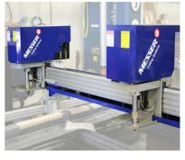
**DUAL MOTORIZED CARRIAGE** Each carriage has it's own servo drive allowing for spacing along independent and cross axis beam. (Optional)
