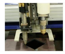
ALFA TORCH Advanced oxyfuel technology with Omniflow automatic gas regulation system and height control. (Optional)
