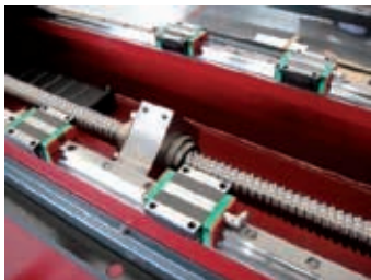
Separate Stainless Steel Tank with Ball Screws motion system with automatic lubrication
