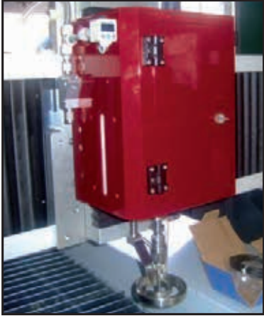
Touch Probe Sensor with Anticollision, Laser Pointer, and Vacuum Assist
