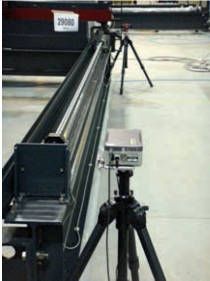
Renishaw Laser Straightness inspection and verification
