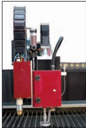
Single Axis with Waterjet and Plasma heads integrated
