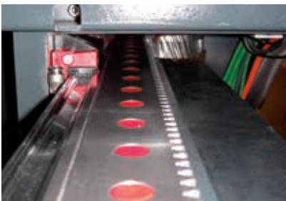
Stainless Steel Tank and 3 axis NC gantry technology with helical rack and pinion motion system with automatic lubrication
