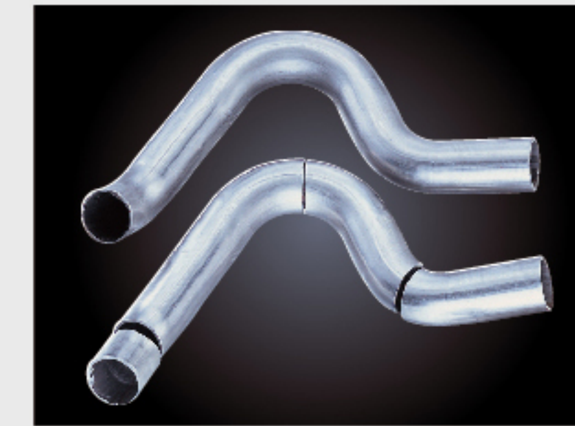
Ø 50.8mm x 1.5t x 1D (Stainless) ( 18% Wall Thinning Control )
