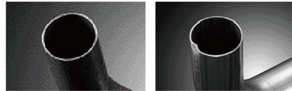
DBS System - Perfect Cutting Face Non-DBS System
