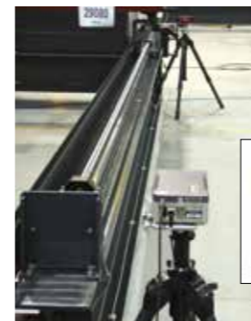
Renishaw Laser Straightness inspection and verification
