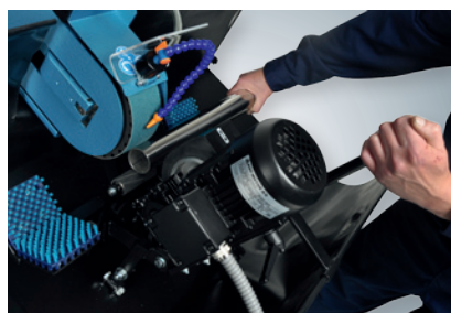
Easy operation - mobile and flexible attachment for Scantool 75 belt grinder.
