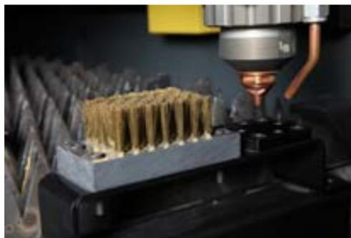
CNC controlled feature allows cleaning and quick calibration of nozzle at predefined numbers of piercing. Applying auto nozzle cleaning avoids problems caused by stacked spatters and ensure height following accuracy.
