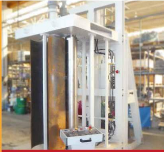
Ahs 4 rolls vertical plate bending machine Ahs 4 valsli dikey silindir makinesi
